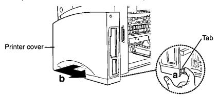
**5** a) Rotate the printer cover away from the printer.**b**)Lift the printer cover away.
