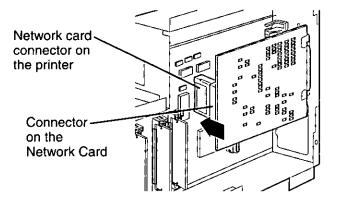
**4** Gently tighten the two screws to secure the Network Card to the printer control board.
