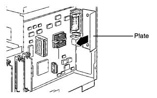
**3** Insert the connector on the Network Card into the network card connector on the printer control board until it is completely in place.
